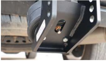
Figure 5: Fill up air bag using the air valve located on the bottom side of the hitch.
