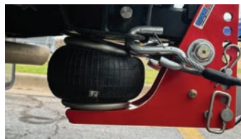
Figure 2: Air bag paddle is showing too much "angle" and needs to be corrected with a paddle spacer block.
