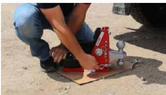
Figure 1: Press in the air valve core and press downward on the air bag paddle to release excess air pressure.
