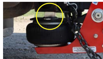
Figure 3: Air bag paddle angle is corrected using the paddle spacer block - only provided with 2" & 2-1/2" HD models.
