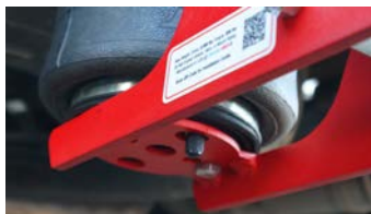
Figure 8: Air hitch up until the main frame makes contact with the "bigger" bump cushion and compresses 1/8"
