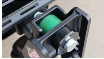
Figure 6: Air hitch up until the main frame makes contact with the "bigger" bump cushion and compresses 1/8"
