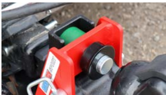
Figure 7: Fill up air bag using the air valve located on the bottom side of the hitch.
