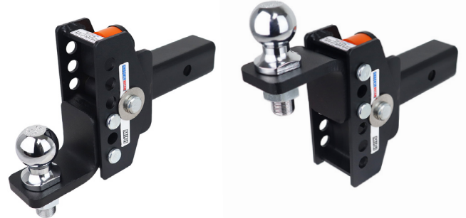
FIGURE 1: ORANGE bushings facing "upward" the weight is on the GREEN bushing - 3,500 lb GTW & 350 lbs TW
