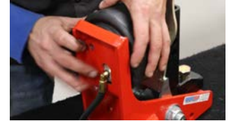
Figure 3: Guide air bag through slotted hole of main hitch frame with the air line facing toward the front.
