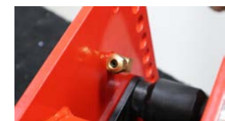
Figure 6: Inner air fitting facing toward the rear of the hitch
