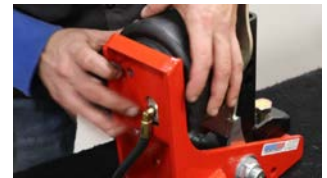
Figure 3: Guide air bag through slotted hole of main hitch frame with the air line facing toward the front.
