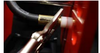
Figure 1: Hold air line with a needle nose pliers to prevent it from spinning during disassembly
