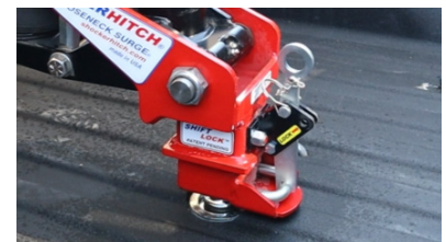
Figure 4: Shift Lock coupler lowered onto gooseneck ball
