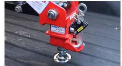
Figure 3: Shift Lock coupler in unlocked position, lower hitch onto gooseneck ball
