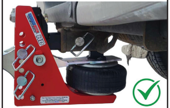
Figure 3: Excessive angle fixed with spacer block
