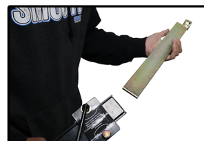
Figure 5: Loosen tension of friction sway arm and remove slide bar
