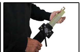
Figure 6: Flip slide bar over and reinsert into friction sway arm unit
