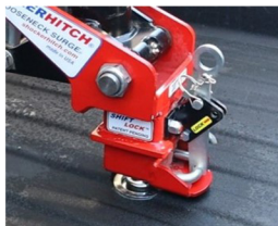
Figure 4: Shift Lock coupler lowered on gooseneck ball
