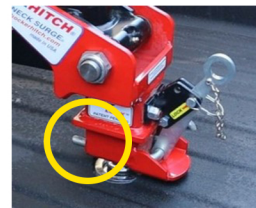
Figure 5: Shift Lock coupler in locked position correctly
