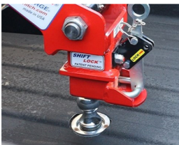
Figure 3: Shift Lock coupler in unlocked position
