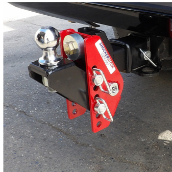
RAISED BALL: 5" RISE TO 3" DROP 2-5/16" BALL - 20,000 LBS/2" BALL - 10,000 LBS
