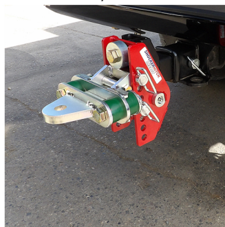
CUSHIONED DRAWBAR: 3.5" RISE TO 3.5" DROP 20,000 LBS
